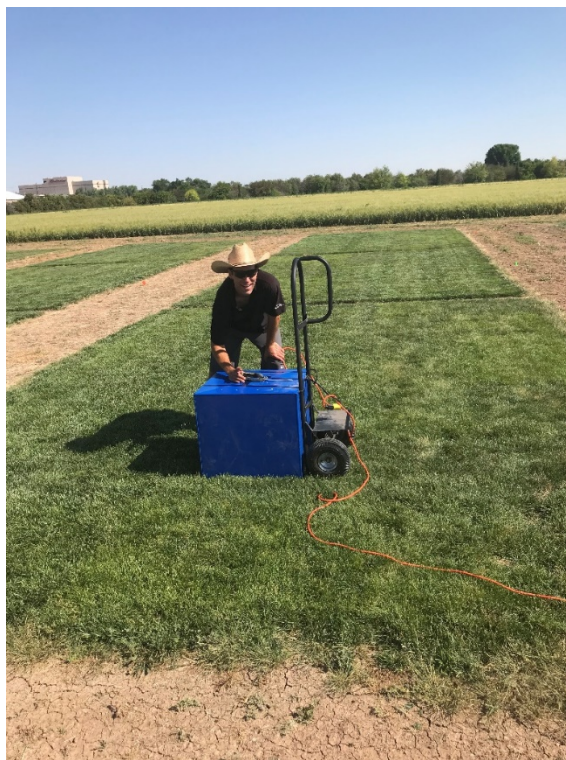
LIGHT BOX UNIT USED TO COLLECT DIGITAL IMAGES OF % GREEN COVER
