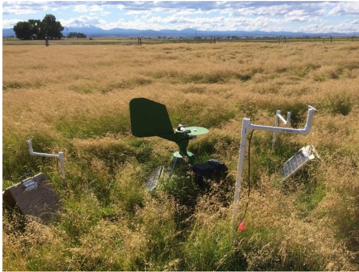
Fig 1. Rotating-arm spore samplers at different sampling heights (2ft, 3ft, and 4ft above the ground) were placed alongside a Burkard spore sampler to collect ergot spores simultaneously in the field.
